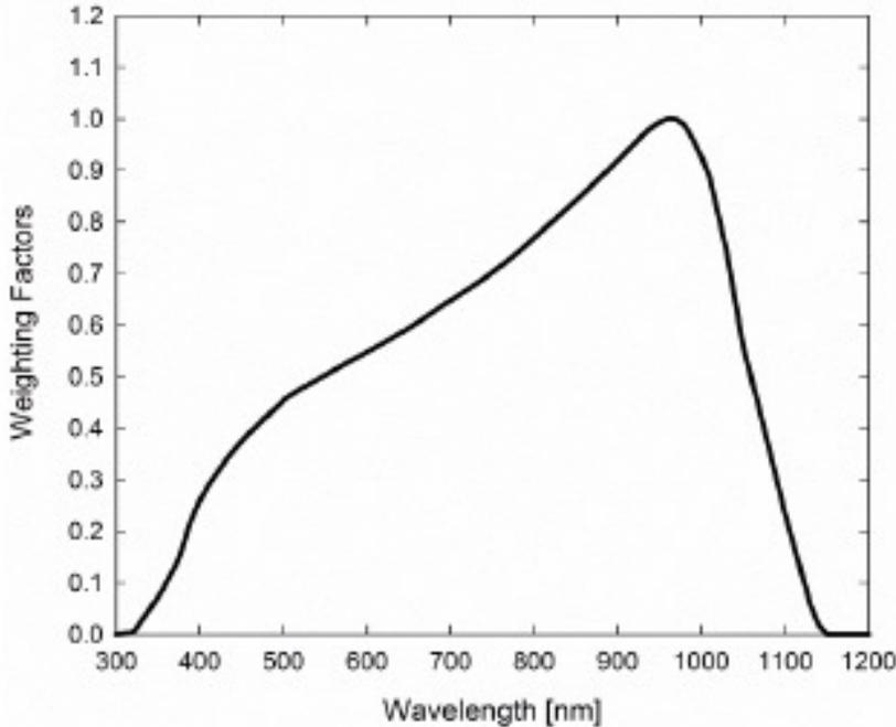
As you can see from the above chart the area of greatest energy is centered in the area of near and far Infrared spectrum which actually is what causes a cabinet surface temperature to rise. The majority of solar energy in the visible spectrum will cause minimal temperature rise.
